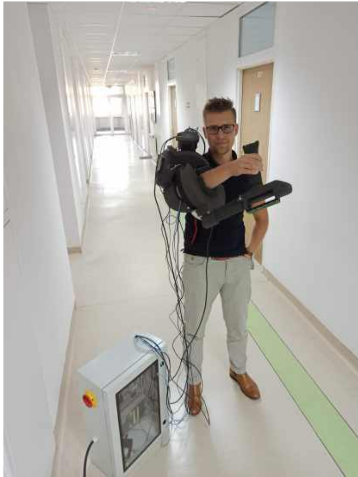
Figure 10: Final prototype of the exoskeleton assembled directly on a user.
