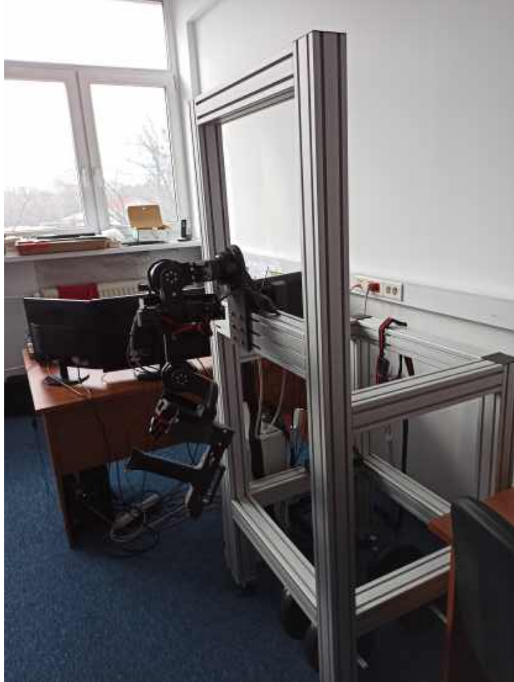
Figure 11: Final prototype of the exoskeleton assembled on a test frame.
