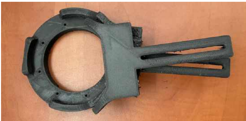
Figure 9: Broken element 3D-printed with FFF technology.
